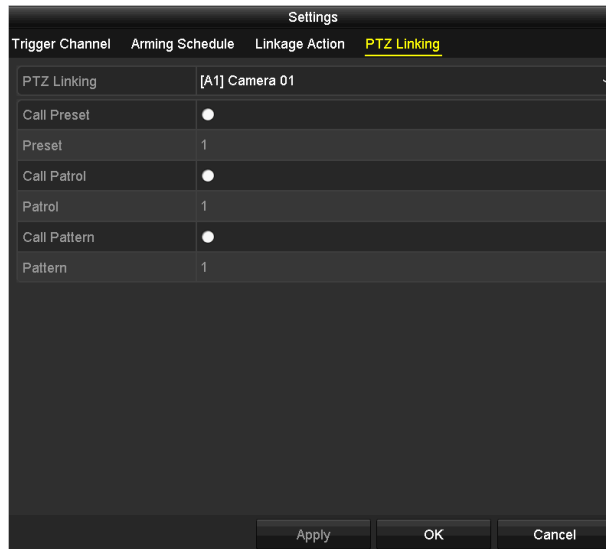
Figure 8-7 Set PTZ Linking of Alarm Input
